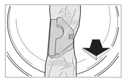
Warning! If the appliance was not transported in an upright position, leave it to stand for 12 hours before connecting it to the electricity supply and using it for the first time, so that the oil can flow back to the compressor. Otherwise the compressor could be damaged.
